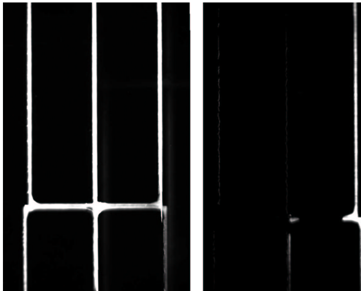
Fig. 4. Fluorescence image of flow in strand transfer module. Flow is from bottom to top and the dye enters on the right channel. Left image: zero flow rate, no separation of solutions. Right image: finite flow rate (see text), no dye in left channel.
